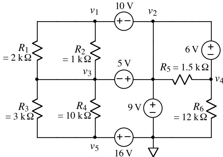
Find the absolute voltages at all the labeled nodes in the above circuit.
