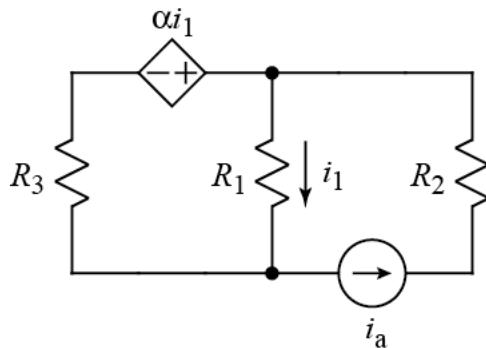
Derive an expression for  $i_1$ . The expression must contain no other parameters than  $i_a$ ,  $R_1$ ,  $R_2$ ,  $R_3$ , and  $\alpha$ . **Note:**  $\alpha < 0$ . (Hint: It is not just a voltage or current divider.)
