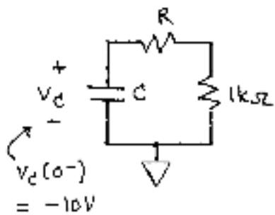
$$v_c(t > t_0) = v_c(t \rightarrow \infty) + [v_c(t_0^+) - v_c(t \rightarrow \infty)] e^{-t/\tau}$$
