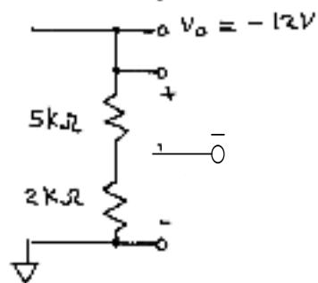
We have a voltage divider:  $v_3 = -12V \cdot \frac{5\text{k}\Omega}{2\text{k}\Omega + 5\text{k}\Omega} = -\frac{60}{7}\text{ V}$ .
