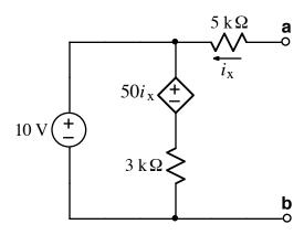
Find the Thevenin equivalent of the above circuit relative to terminals **a** and **b**.
