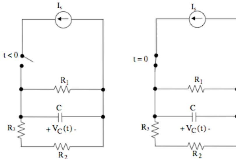
After being open for a long time, the switch closes at  $t = 0$ . Write an expression for  $v_C(t > 0)$  in terms of at most circuit quantities  $R_1$ ,  $R_2$ ,  $R_3$ ,  $i_s$ , and  $C$ .
