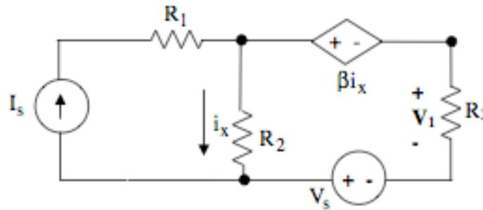
Using superposition, derive an expression for  $v_1$  that contains no circuit quantities other than  $i_s$ ,  $v_s$ ,  $R_1$ ,  $R_2$ ,  $R_3$ , and  $\beta$ , where  $\beta < 0$ .
