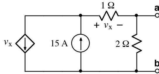
Find the Thevenin equivalent of the above circuit relative to terminals **a** and **b**.
