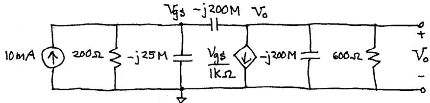
Using exact Node-Voltage method:
