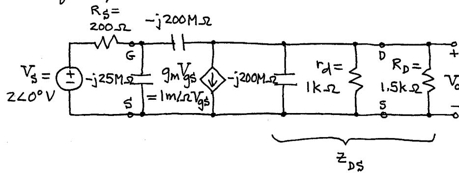
$$z_{DS} = -j 200M \parallel 1k\Omega \parallel 1.5k\Omega$$
