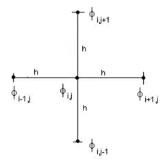
$$\nabla^2 \phi = \frac{\partial^2 \phi}{\partial x^2} + \frac{\partial^2 \phi}{\partial y^2} = 0$$
