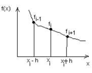
$\begin{aligned} f'(x_i + h/2) &= (f_{i+1} - f_i) / h + error ((h^2/6) f''') \\ f'(x_i - h/2) &= (f_i - f_{i-1}) / h + error ((h^2/6) f''') \\ f''(x_i) &= (f'(x_i + h/2) - f'(x_i - h/2)) / h \\ &= (f_{i+1} - 2f_i + f_{i-1}) / h^2 + error ((h^2/3) f''') \end{aligned}$
