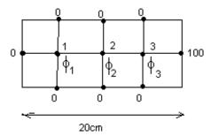
h=20 cm / 4 divisions = 5 cm = 0.05 meters 3. Apply Difference Equation at Each Node (1,2,3) Node 1:  $[0+0+0+P2 - 4*P1] / 0.05^2 = 0$ Node 2:  $[P1+0+0+P3-4*P2] / 0.05^2 = 0$ Node 3:  $[P2+100+0+0-4*P3] / 0.05^2 = 0$  (Multiply through by  $0.05^2$ )
