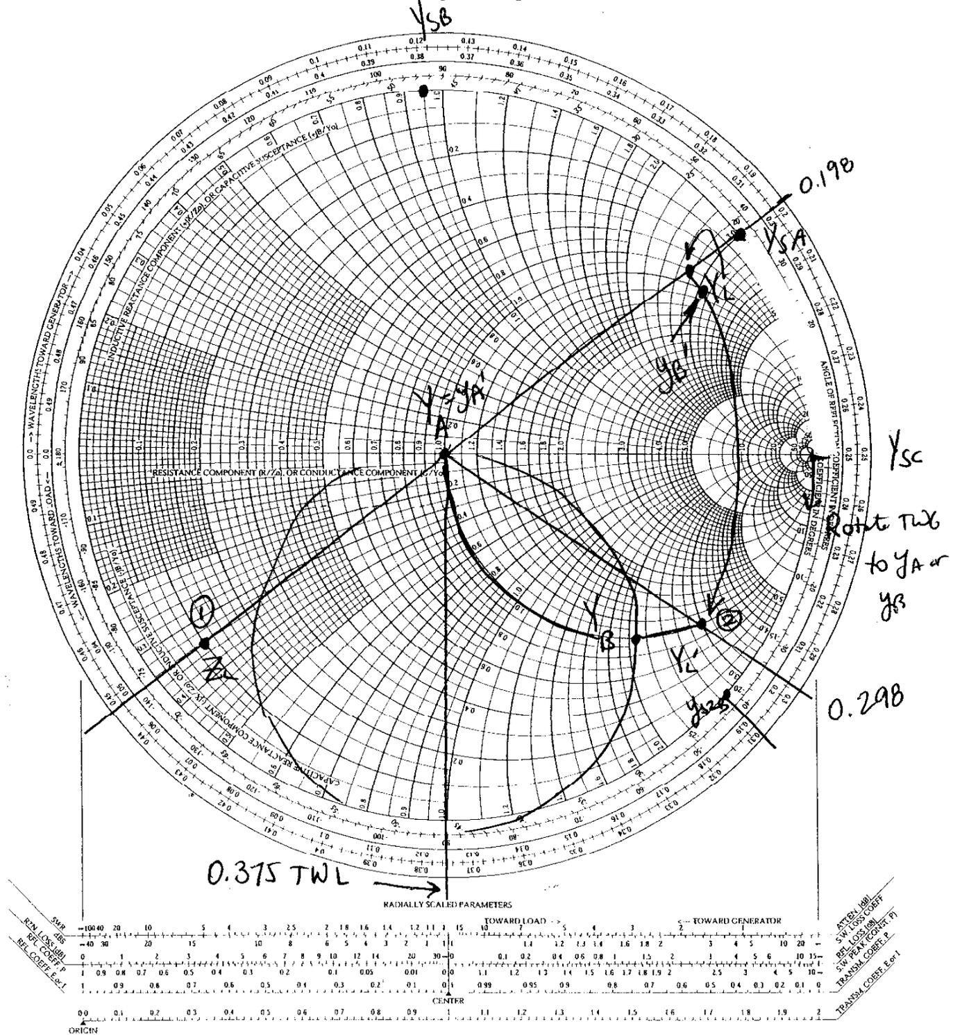
3. (20 points) Design an L matching network to match a load of  $Z_L = 100$  ohms to a 25 ohm line. Specify the value of all capacitors and inductors to make this a low pass configuration. (Assume  $f = 1\text{MHz}$ )
