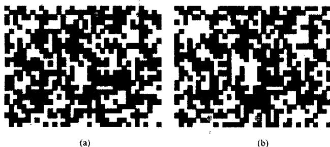
Fig. 7. Feed and ground locations: the dimensions of (a) the GA antenna with constraint varying feed and ground and constraint P(L) > P(W) and (b) the GA antenna without the constraints.
