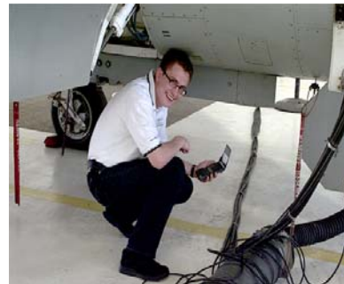
PICTURE 6: The modified BT Palm Pilot receiving temperature data. (Jens Hult ) - Specialist Engineer
