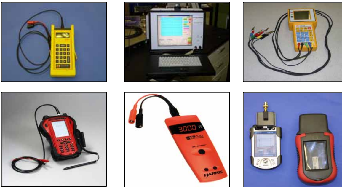
Figure 7. Handheld or portable wiring diagnostic technologies evaluated
