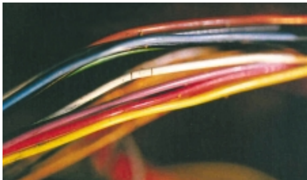
Wiring taken from U.S. Navy aircraft show [left] cracks in the polyimide insulation that go through to the copper conductor, and [right] faults in PVC-insulated wire that had been hidden under a clamp; the discoloration indicates arcing had occurred.
