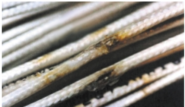
Wiring taken from U.S. Navy aircraft show [left] cracks in the polyimide insulation that go through to the copper conductor, and [right] faults in PVC-insulated wire that had been hidden under a clamp; the discoloration indicates arcing had occurred.
