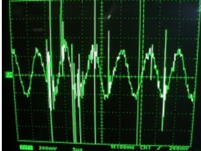
Figure 6. The output from the oscilloscope that shows noise being generated along the power line in the parallel configuration by a switching action. The frequency of the generated noise was found to be around 30 MHz.
