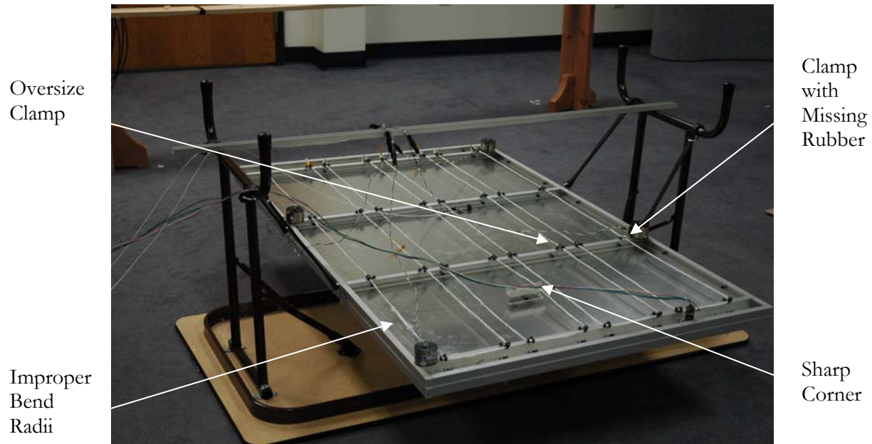
Figure 13 – Test panel 1 harness anomalies.
