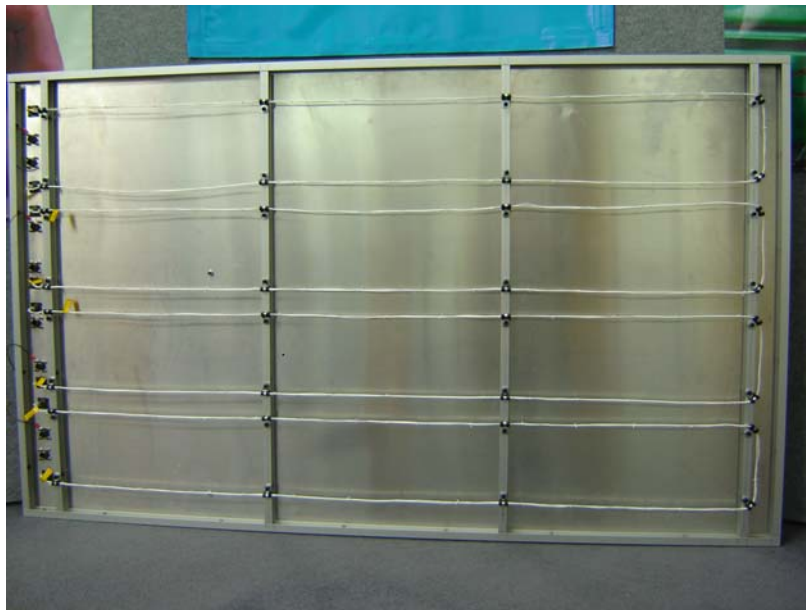
Figure 4 – Test panel showing properly run harnesses.
