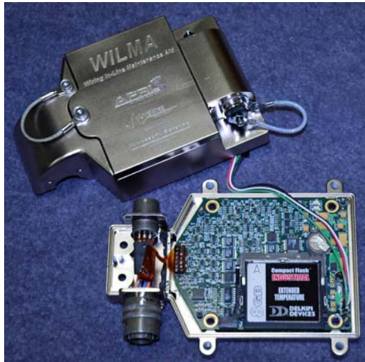
Figure 3 Prototype implementation of the S/SSTDR Tester or WILMA.
