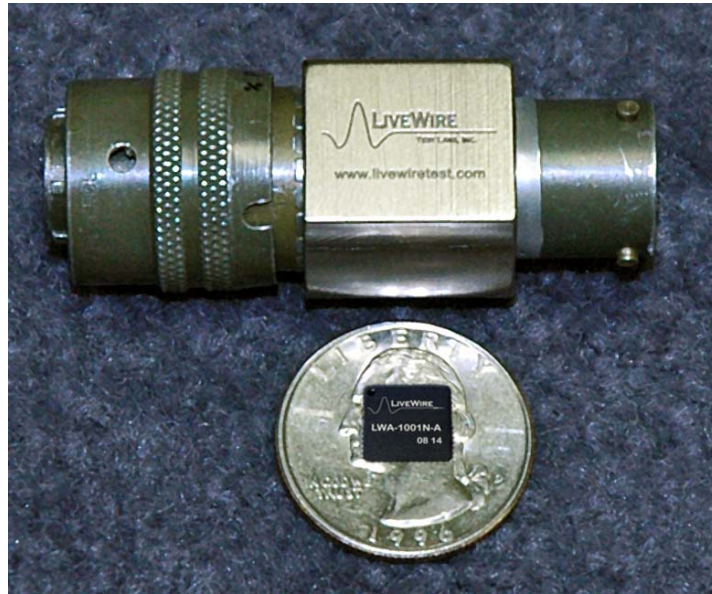
Figure 6 Size comparison with “Smart Connector” and LiveWire SSTDR ASIC
