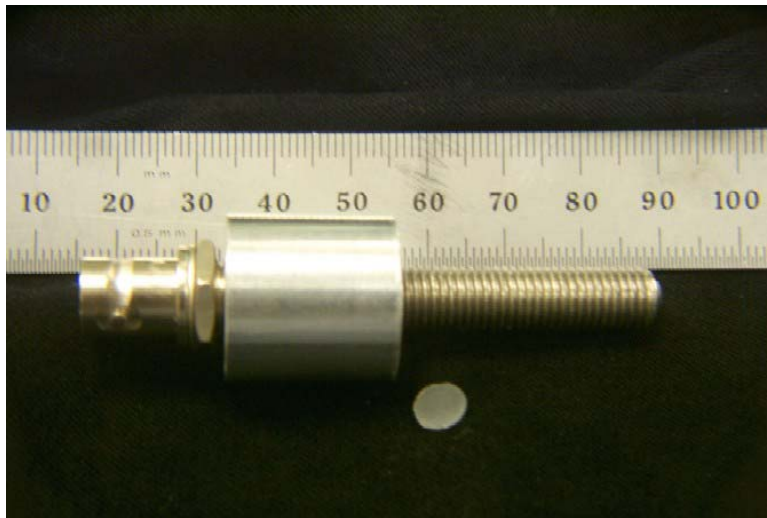
Figure 8. Arc test fixture assembled.
