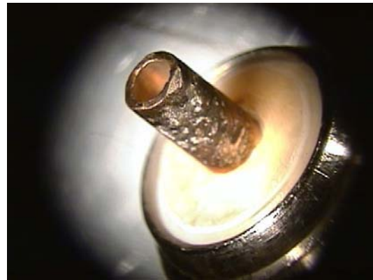
Figure 57. BNC connector pin located in the arc test fixture.
