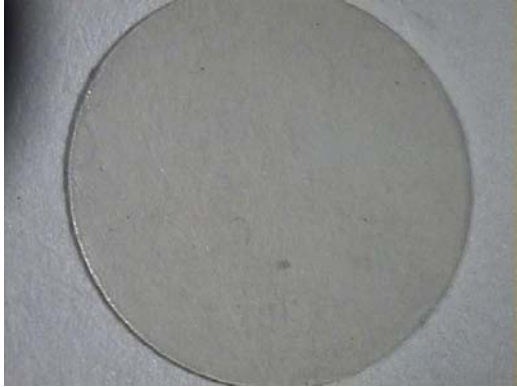
Figure 51. Microscopic photograph of a mylar sample before a low energy breakdown.
