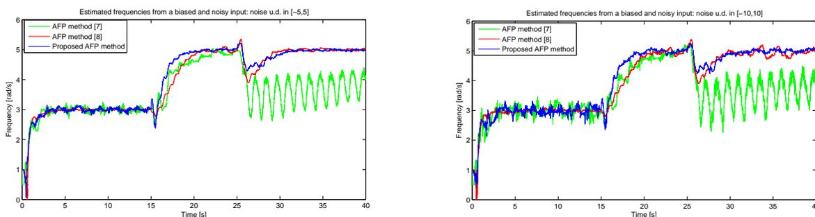
Fig. 3. Time-behavior of the estimated frequency by using the proposed AFP method (blue line) compared with the time behaviors of the estimated frequency by the AFP methods [8] (red line) and [7] (green line), respectively. a)  $d(t)$  random noise with uniform distribution in the interval  $[-5, 5]$ ; b)  $d(t)$  random noise with uniform distribution in the interval  $[-10, 10]$ .
