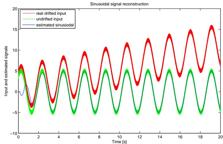
Fig. 5. Estimated sinusoidal signal by the proposed AFP method.
