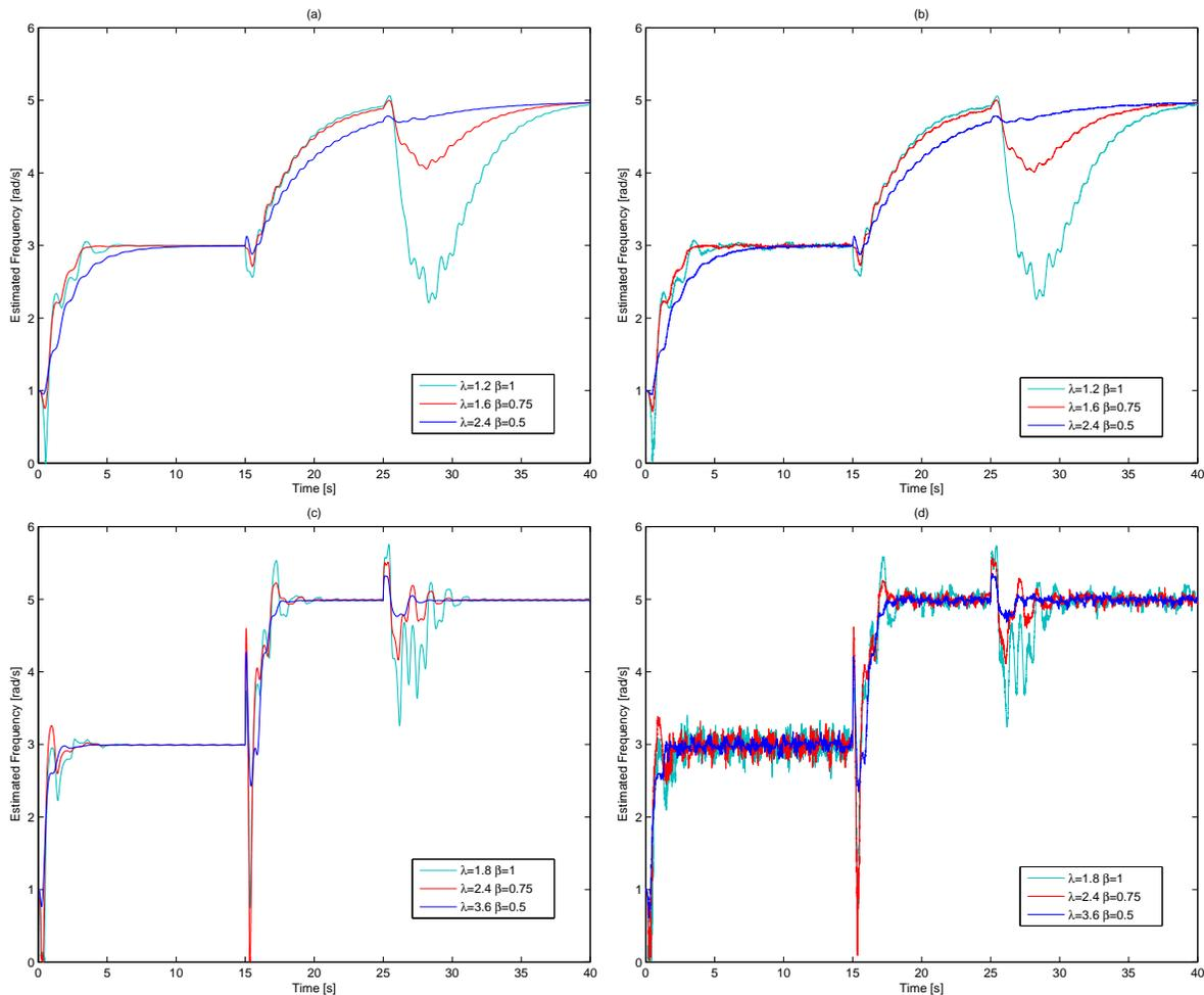
Fig. 4. (a) Estimated frequencies without unstructured noise and (b) with random noise  $d(t)$  uniformly distributed in the interval  $[-2.5, 2.5]$  using different values of  $\lambda$  and  $\beta$  such that  $\lambda\beta = 1.2$ . (c) and (d) Same as for (a) and (b) with  $\lambda\beta = 1.8$ .
