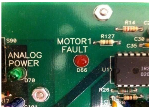
Figure 7(a): Motor-1 Fault Indicator
