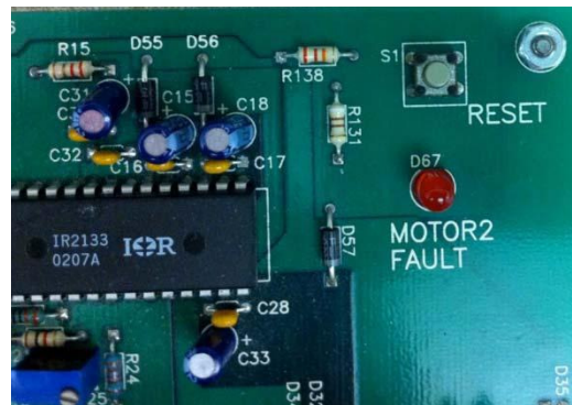
Figure 7(b): Motor -2 Fault and Reset Switch
