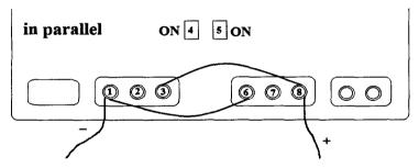
(2) When the two ways power supply are in parallel, the voltage regulation knob (17) and current regulation knob (18) of the subordinate power supply will not work. Regulate the knob (13), the output voltage of the subordinate trace the main output voltage, the output voltage value is that of main. Regulate the knob (14), the
