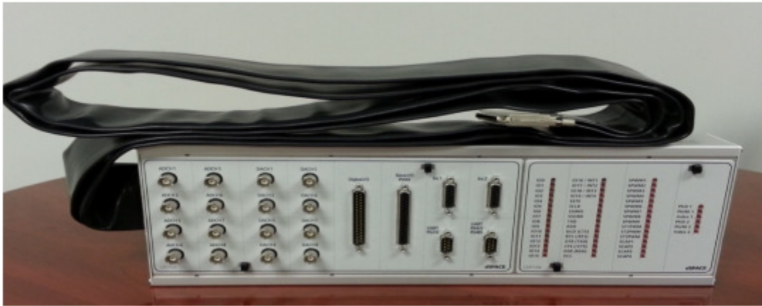
Figure 3: CP 1104 I/O box with attached master I/O ribbon
