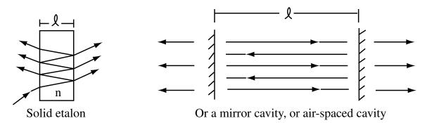
setting the refractive index n = 1. The air-spaced cavity is essentially a laser cavity, or open resonator.
