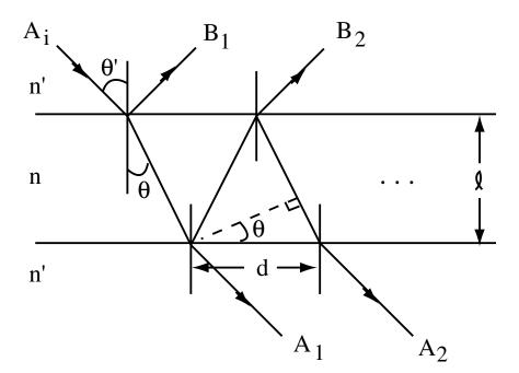
Now, the relative phase shifts  $\phi$  between rays  $B_1$  and  $B_2$ , and between  $A_1$  and  $A_2$  need to be included. The phase  $\phi$  is due to the extra path length inside the etalon for each component of the wavefront. In the figure
