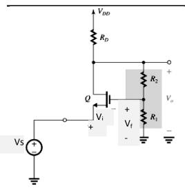
Open-loop gain: without  $R_2$  and  $R_1$  ang the gate grounded:  $V_O = -g_m V_{gs} \times R_D$  $V_{gs} = -V_S \Rightarrow A = g_m R_D$ Feed-back factor:  $\beta = \frac{V_f}{V_0} \Rightarrow V_f = \frac{R_1}{R_1 + R_2} \cdot V_0 \Rightarrow \beta = \frac{R_1}{R_1 + R_2}$
